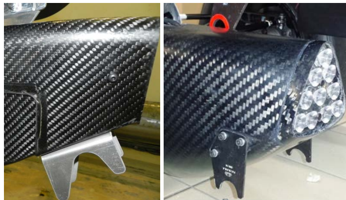
Figure 1. Example of an aggressive shaped jacking point
