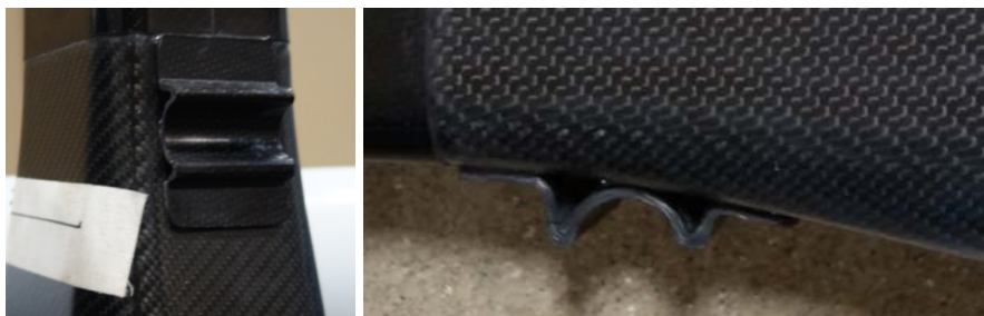
Figure 2. Example of a less aggressive jacking point design
